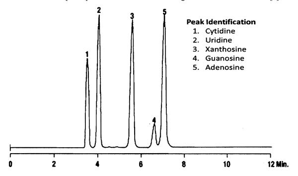
Figure 1: HPLC chromatogram for a mixture of nucleosides
