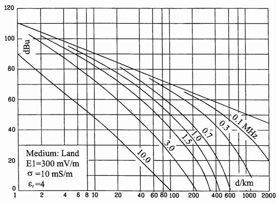
Figure 4 Ground propagation paths
