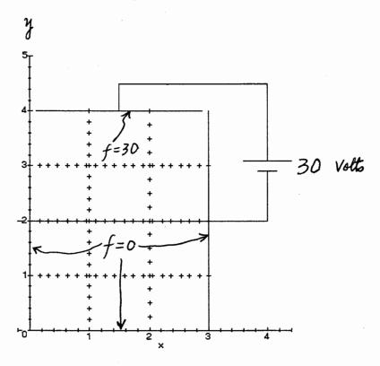
The boundary conditions are given as f(0,y) = 0, f(3,y) = 0, f(x,0) = 0 and f(x,4) = 30 volts. Use the discrete Laplace equation, i.e.,
