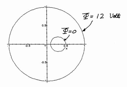
The outer cylinder has a radius of unity and centered at the origin while the inner one has a radius of 0.2 and centered at (0.3, 0).
