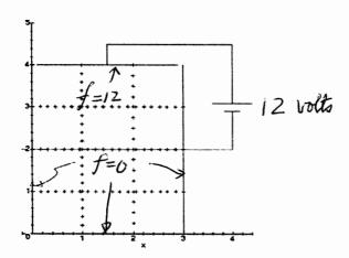
The Dirichlet boundary conditions are given as f(0,y) = 0, f(3,y) = 0, f(x,0) = 0 and f(x,4) = 12 volts.
