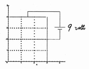
The Dirichlet boundary conditions are given as f(0,y) = 0, f(3,y) = 0, f(x,0) = 0 and f(x,4) = 9 volts.
