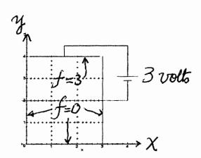
The Dirichlet boundary conditions are given as f(0, y) = 0, f(3, y) = 0, f(x,0) = 0 and f(x,4) = 3 volts.
