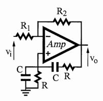
Q5b: Discuss the stability of the amplifier in terms of the resistor ratio,  $R_2/R_1$   $\equiv \eta$ ; that is, to discuss circuit states in every possible domain  $(\eta_i, \eta_{i+1})$  in  $[0,\infty)$ . 10 pts
