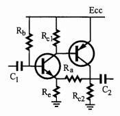
Q3b: Calculate the voltage amplification factors both with and without feedback. Given signal source:  $R_s$ =0; Circuit components in Ohm:  $R_{C1}$ = 8K,  $R_{C2}$ =2K,  $R_e$ =0.2K,  $R_a$ =8K. Be aware that the second transistor is pnp but complimentary to the first; ie, the two are identical in their parameters,  $r_{\pi}$ =2K Ohm,  $\beta$ =120. Needs symbolic network equations first before numerical solving calculation. 10 pts (5 pts for with, 5 pts for without)
