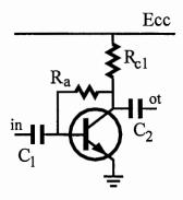
Q3b: Calculate the voltage amplification factors to Es, ie, Av=Vo/Es, both with and without feedback. Given signal source:  $R_s=1$  KOhm;  $R_{C1}=2K$ ,  $R_a=20K$  and C1, C2 large. The transistor parameters are:  $r_\pi=2K$  Ohm,  $\beta=120$ . Needs symbolic network equations first before numerical solving calculation. 10 pts (5 pts for with, 5 pts for without)
