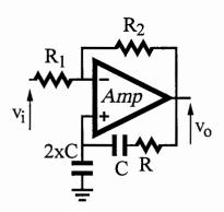
Q5b: Discuss the stability of the amplifier in terms of the resistor ratio,  $R_2/R_1$   $\equiv \eta$ ; that is, to discuss circuit states in every possible domain  $(\eta_i, \eta_{i+1})$ .
