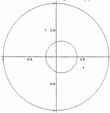
The outer cylinder has a radius of unity and centered at the origin while the inner one has a radius of 0.3 and centered at (0.1, 0).
