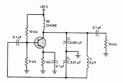
If the value of L is doubled in the figure above, what will be the frequency of oscillation? (4)
