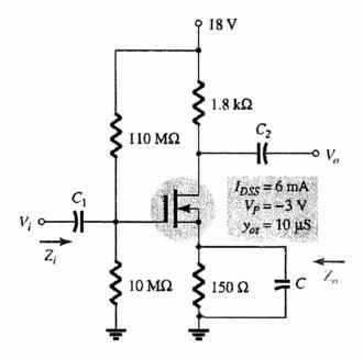
a) Determine  $g_m$ . (4) b) Find  $r_d$ . (1) c) Draw the ac small signal equivalent network for the above circuit. (5) d) Find  $Z_i$ . (5) e) Find  $Z_o$ . (5)
