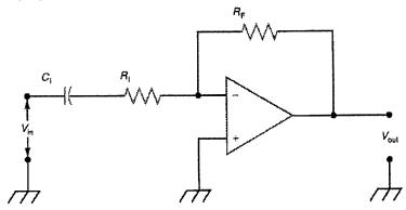
where  $R_i = 2k\Omega$ ,  $C_i = 0.1 \mu F$ ,  $R_F = 100 k\Omega$ .
