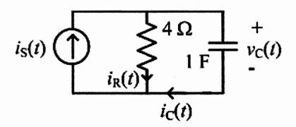
For the circuit shown above, use Laplace transforms to find the steady-state response at  $v_C(t)$  when  $i_S(t) = \cos(t)u(t)$ . (10)
