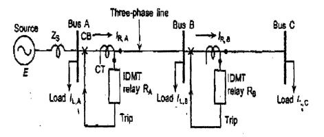
a) Determine the CT ratios and the plug settings for the relays at bus A and bus B. Assume 20% overload when calculating the maximum load, 2 A relay rating is used and the plug settings to be done at 100%. Note: Assume the available CT ratings are: 100 A, 200 A, 300 A, 400 A, 500 A, 600 A ......,etc
