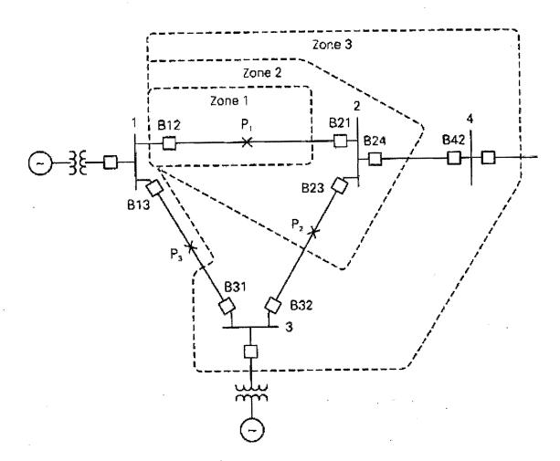
a) Determine the three impedance relay zones settings at breaker B12  $Z_{r1}$ ,  $Z_{r2}$ ,  $Z_{r3}$ , and time delay for the relay to trip in each zone.
