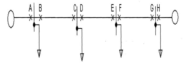
If there is a fault in the middle of the line FG, which relays are going to energize and what will be their operating time acceding to your coordination?
