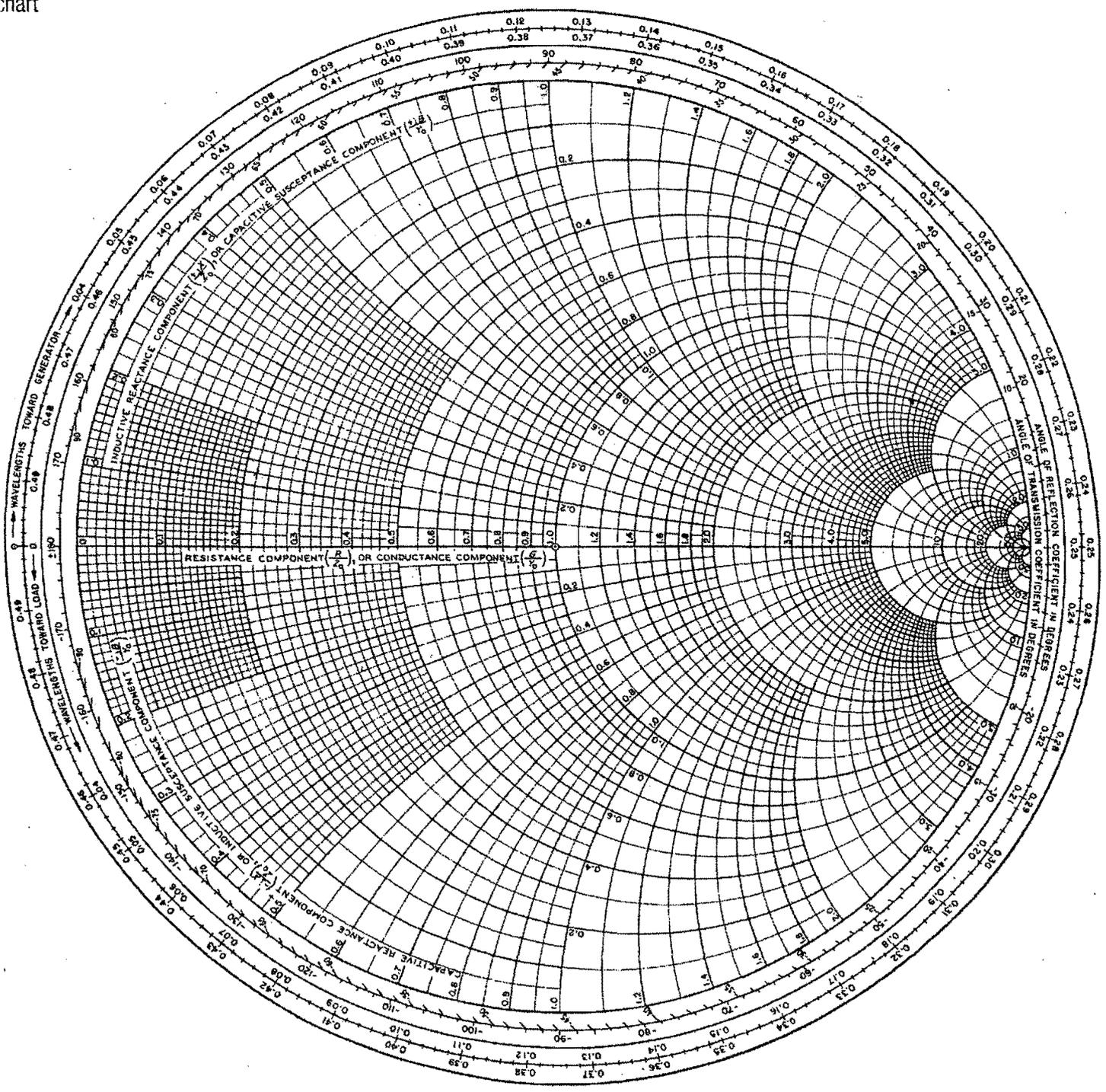
**Q4: (20 pts)** A lossless TV transmission line of  $75 \Omega$  feeds a dipole antenna of impedance  $70+j40 \Omega$ . (i)(5 pts). Find VSWR. To improve the VSWR design a  $\lambda/4$  transformer inserted in somewhere in the transmission from the load, (ii)(10 pts). Calculate the location from the load to put the  $\lambda/4$  transformer, (iii)(5 pts). the  $Z_o$  of the transformer.
